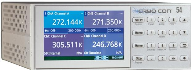
The model 54 is a next generation four-channel cryogenic impedance bridge capable of measuring resistance, inductance and mutual-inductance. Additionally, four control loop outputs support use as a temperature controller.
