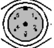
**Note:** The input connectors on the Model 32 will mate with either DIN-5 or DIN-6 plugs. Wiring is identical. If a DIN-6 plug is used, Pin 6 is not connected.
